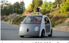
possible with a foam bumper and a flexible windscreen that is designed to absorb energy from an impact with a person's body.
